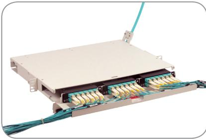
The AFL 1RU Fiber Termination Patch/Splice Panel is designed for use as a rack mount interconnect point where termination and connectivity of up to 36 fibers is desired. The panel design is based on a 1 rack unit height and is provisioned with three LGX® 118 compatible mounting positions that can accommodate adapter plates, XFM® optical cassettes, passive optical modules or any combination therein.
